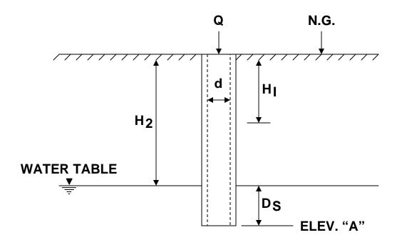
$$K = \frac{4Q}{\pi d (2H_2^2 + 4H_2D_S + H_2d)}$$
